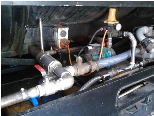
Work on the output piping from the fresh water tank on the service wagon which is used to top up the boiler on Wa165, has been completed. Also a new visual water level pipe was fitted to easily see how much water is in the tank – it was getting a little difficult to see the water level in the old one!
