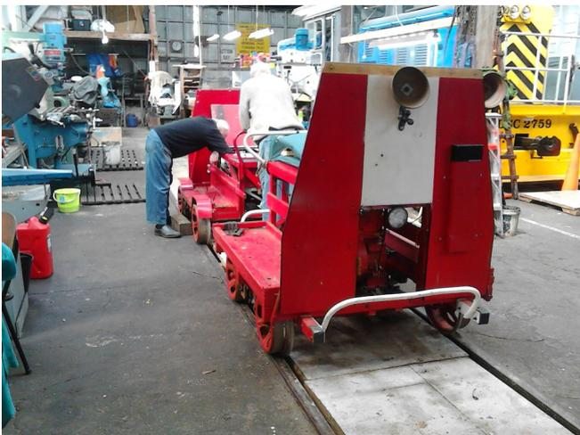
During the weekend it was found to be rather hard to get the engine started and various amounts of black and white smoke were observed coming out of the exhaust. It has been returned to the company which fitted the replacement engine to have more work done on it.
