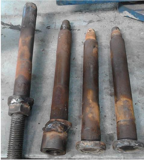
The first pin (in the photo on the previous page) came out relatively easily, but removing the other old, rusty, non-lubricated pins proved to be a real challenge.
