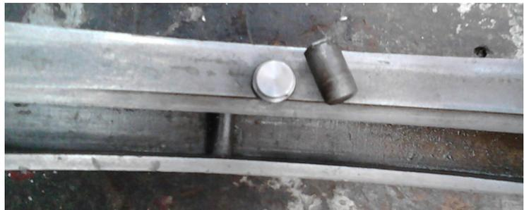
Further inspection revealed that another two complete dust guards (out of the eight normally installed) were missing, allowing dust and dirt etc. into the traction motors. We need to obtain replacement items.
