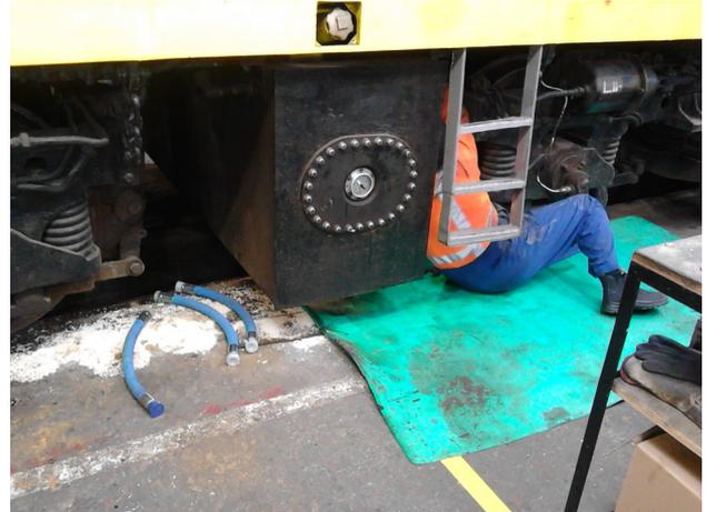
An “interesting” point about the thinking of NZR (as it was then) is that due to the size of the fittings, 1250psi hose has to be fitted, even though only 100psi pressure is required. The 1250psi hose is of course dearer than 100psi hose!
