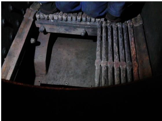
Firstly, to make it easier to work inside the fire box, the fire bars (which co-incidentally Geoff had previously cleaned) were refitted.
