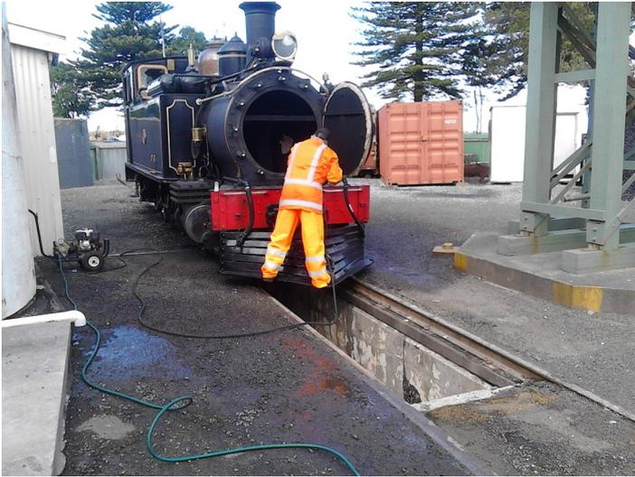
The interior of the boiler has also been water-blasted using an extension rod to spray the water into the boiler through the (removed) boiler plug holes.
