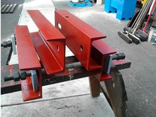
Spotted recently were these "timber clamps" being manufactured in accordance with approved engineering drawings to be fitted as part of the bridge maintenance over the Winter period.
