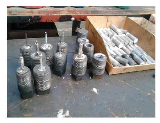
These sacrificial anodes help combat internal chemical deterioration of the boiler.
